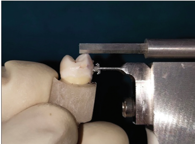
Figure 11: Force sensing blade snugly seats into the bracket slot with vertical stopper passively in contact with cuspal tip.
