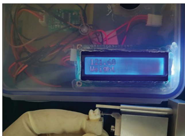
Figure 10: Force sensing blade present inside the bracket slot with bonding force of 121 grams seen in display.
