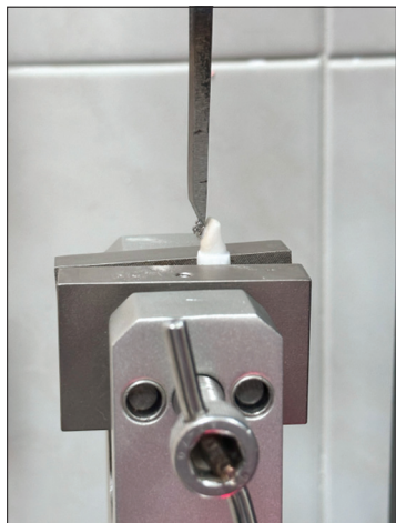
Figure 6: Shear bonding strength measurement by universal testing machine.
