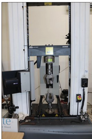
Figure 4: Frictional resistance test using a universal testing machine.
