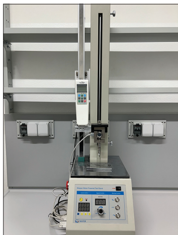
Figure 1: Motorized vertical testing bench TVO-S (AstraLab, Mariano Comense, Italy).
