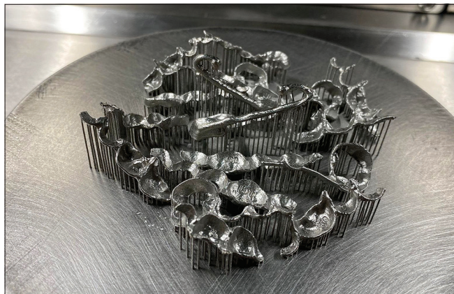
Figure 6: An example of printed orthodontic appliances for clinical application with support structures using selective laser melting technique.
