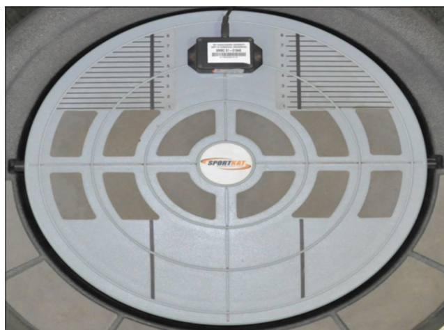
Figure 2: Circular balance platform with two-axis electrolytic tilt sensor
