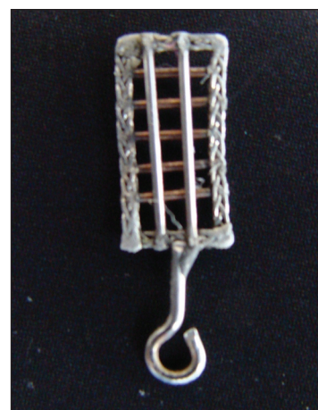
Figure 3: Grid with a hook soldered on to it
