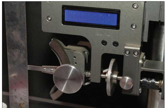
Figure 9: Verifying the accuracy of the torque angulation device using the orientation guide
