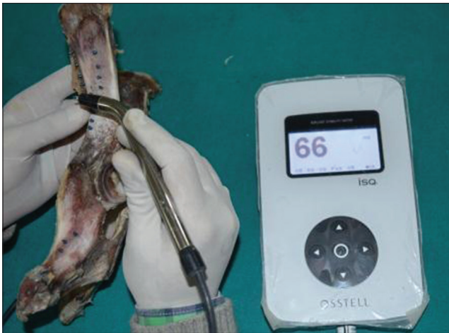
Figure 9: Primary stability measured using Osstell resonance frequency analysis device
