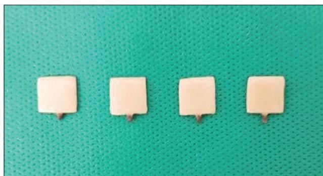
**Figure 1:** Porcelain samples before bonding orthodontic brackets.
