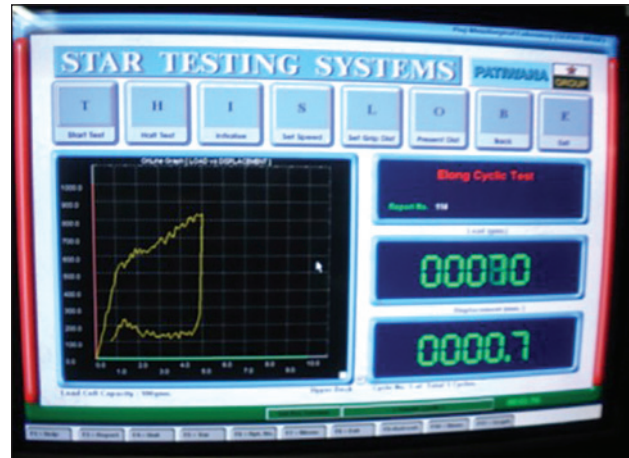
Figure 3: Screenshot of computerized plotting of the load – deflection curve – unloading
