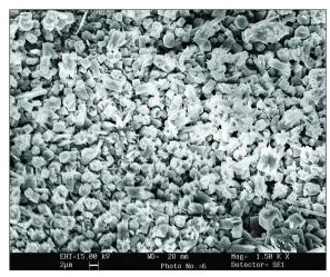
Figure 2: Scanning electron microscope view of etched porcelain
