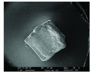
Figure 6: Ceramic bracket representing cohesive failure within adhesive
