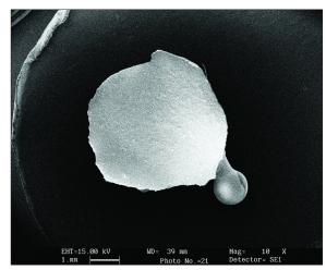
Figure 5: Metal bracket representing adhesive failure at porcelain-adhesive interface
