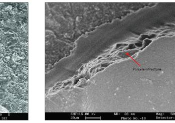
Figure 3: Cohesive failures within adhesive
