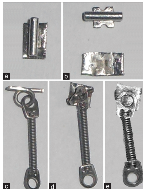
Figure 1: (a) Begg bondable tube. (b) Mesh base. (c) NiTi closed coil spring with steel loop. (d) Spring with welded loop. (e) Spring with eyelet welding
