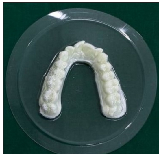
Figure 2: Thermoformed aligner sheets on the crowding model.
