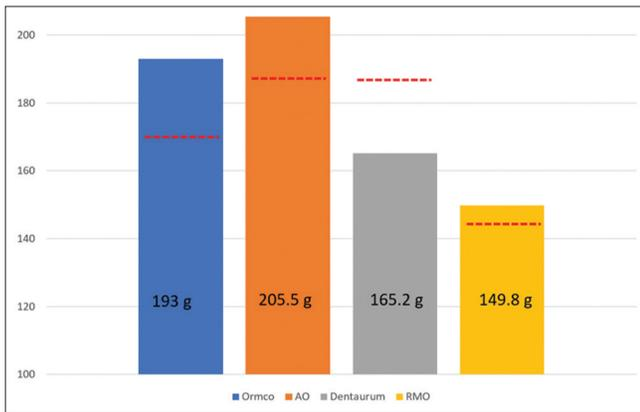
**Figure 3:** Comparison graphs of recorded mean force level at 3 times the lumen size extension with force levels on packs stated by manufacturers for heavy elastics. Dashed lines represent the force levels stated by manufacturers.
