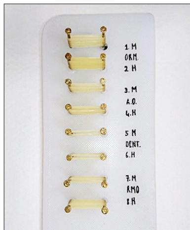
**Figure 1:** The latex elastics placed on the mechanism with screws at a standard 22.3 mm distance.
