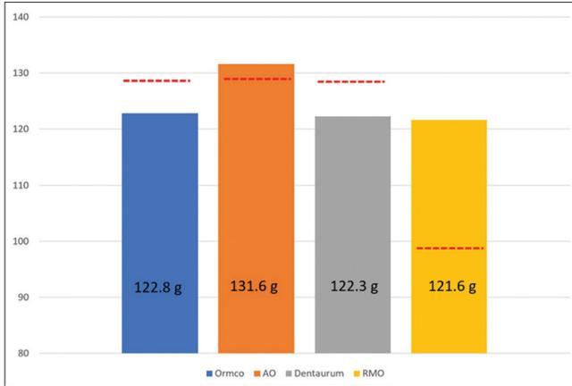
**Figure 2:** Comparison graphs of recorded mean force level at 3 times the lumen size extension with force levels on packs stated by manufacturers for medium elastics. Dashed lines represent the force levels stated by manufacturers.
